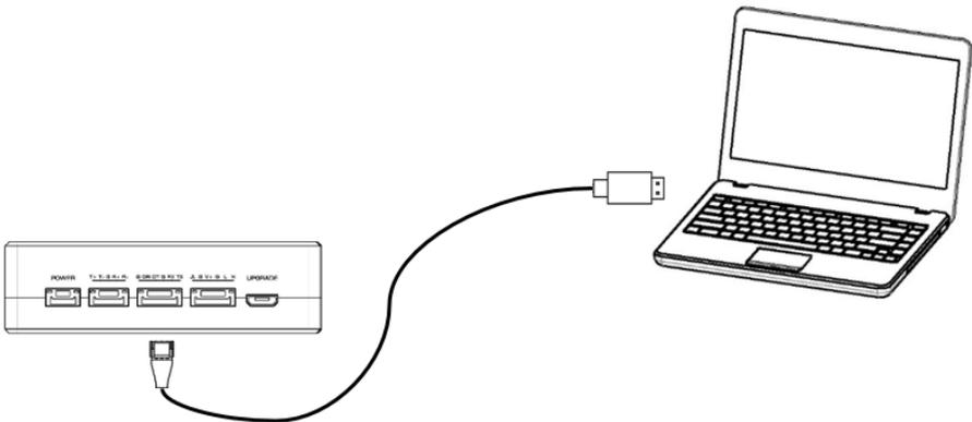
Insert the six-pin connector of supplied serial cable to the serial port of the ground unit and connect the other end of supplied serial cable to the telemetry port of the ground control station.
