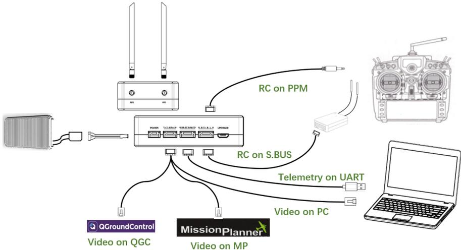
1. Connect antennas to RF ports of the ground unit.
