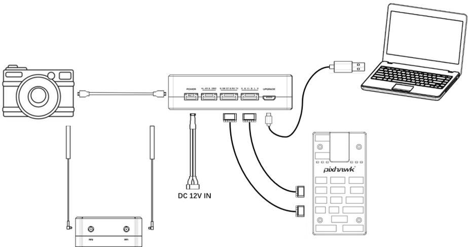
1. Connect antennas to RF ports of the air unit.
