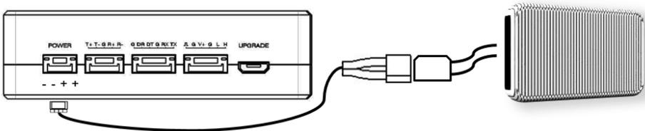
Insert the four-pin connector of supplied power cable to the power port of the ground unit and connect the orange power connect of supplied power cable to a battery output, or can be from a power adaptor. Recommended voltage is 12V.
