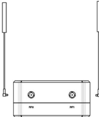
Insert the air unit antennas into the RF ports. Antenna clicks in when properly installed.
