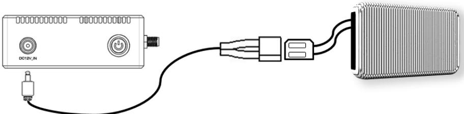
Insert the power connector of the power adaptor into the charging port of the ground unit and insert into the aerial plug into an electrical outlet to fully charge the battery of ground unit. Recommended voltage is 12V.
