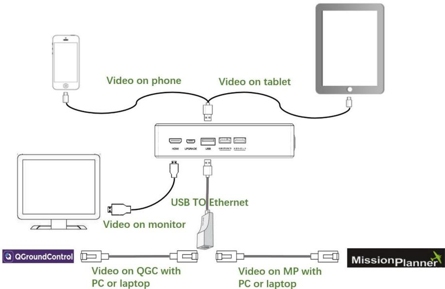
The ground unit outputs video to the monitor via HDMI cable, or you can connect the ground unit to the mobile phone or tablet via USB cable, and opens Viulinx APP to watch the video. QGC is also supported.
