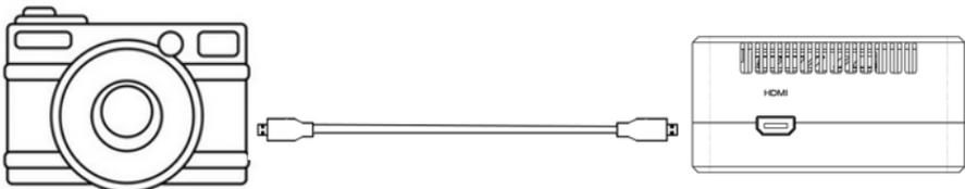
Connect the HDMI video output port to the HDMI video input port of the air unit.
