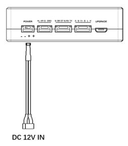
Pin-out: - - + +. Insert the four-pin connector of supplied power cable to the power port of the air unit and connect the orange power connect of supplied power cable to a battery output, or the power supply port of a drone. Recommended voltage is 12V.
