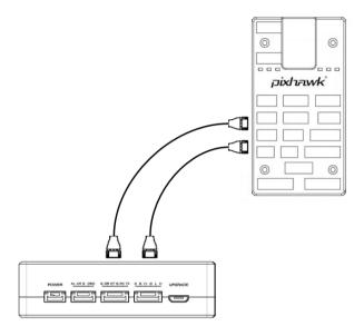
Insert the six-pin connector of supplied serial cable to the serial port of the air unit and connect the other end of the serial cable to the telemetry port of a flight controller.
